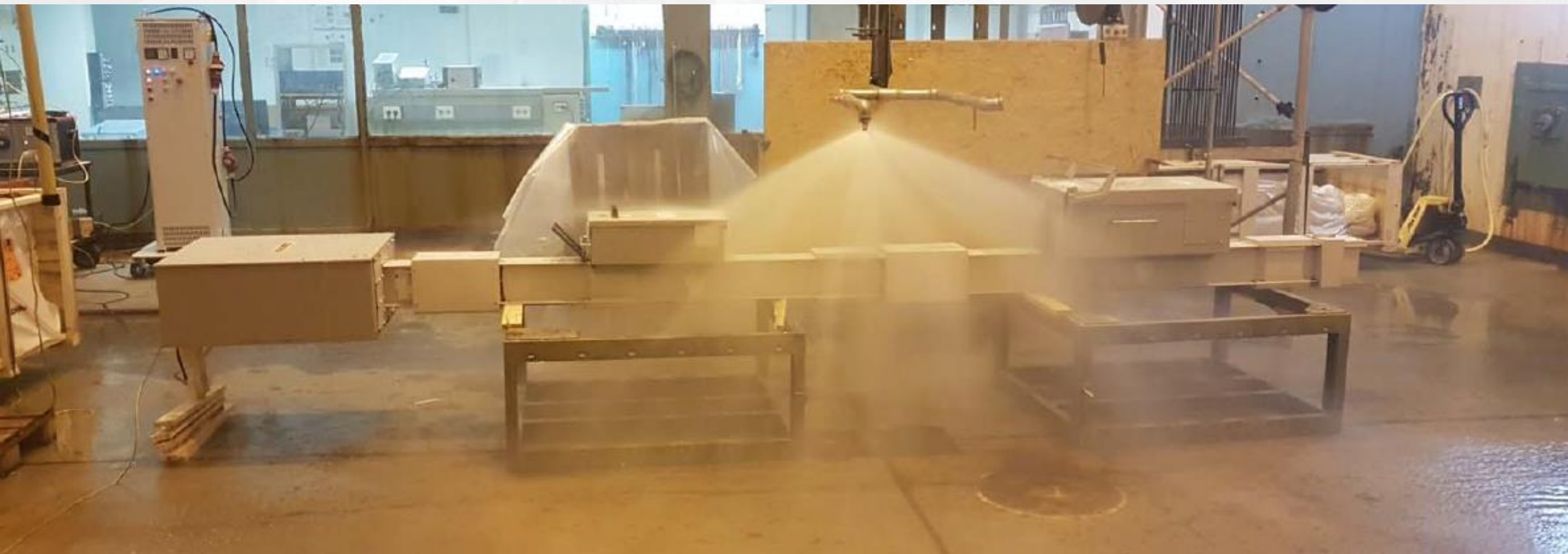
Photo 1: Device under test at 7,5 bar (15 min, approximately 330 l/min)
